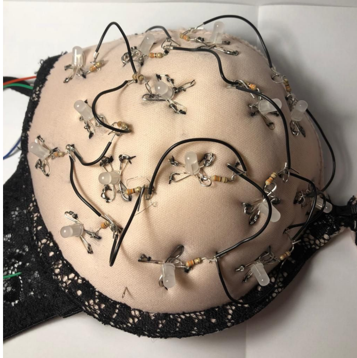
One wire to connect all resistor ground in a series
