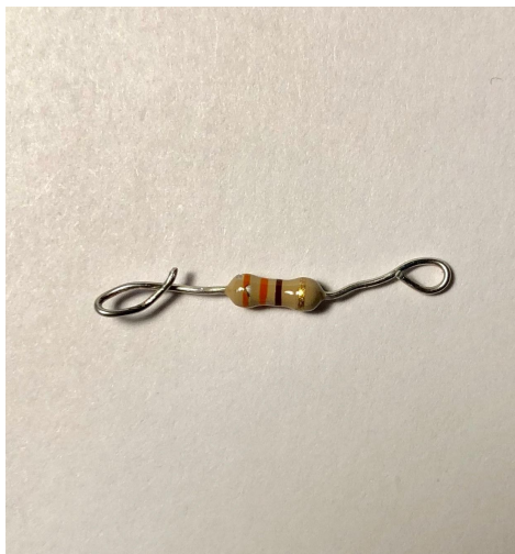
Legs of resistor bent into a loop
